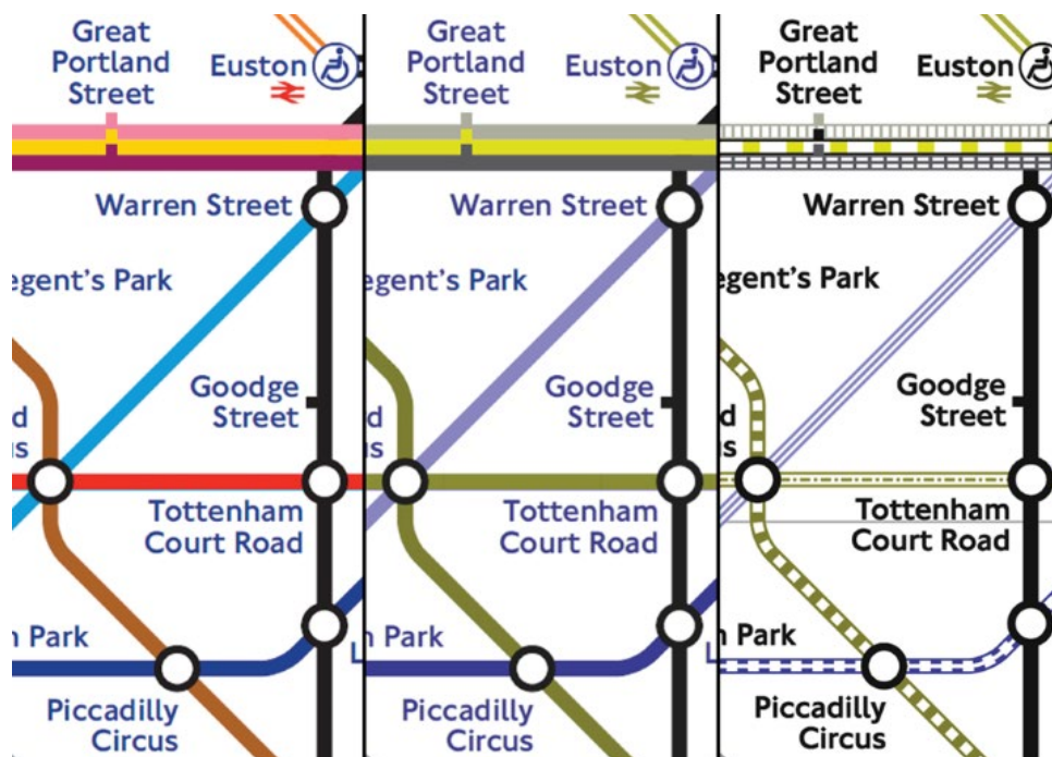
Figure 62. Ian Hamilton. Example of the London underground map viewed with red green colour blindness and the improvement of makings to help differentiate the tube lines 2019.www.brilliantmaps.com
