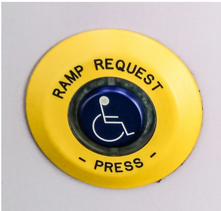
Figure 73. View of disabled ramp request bell that alerts the driver a disabled person wishes to come aboard the bus of a 2017 Routmaster bus, Brighton and Hove Bus depot. Personal photograph by Author.01 Nov.2019
