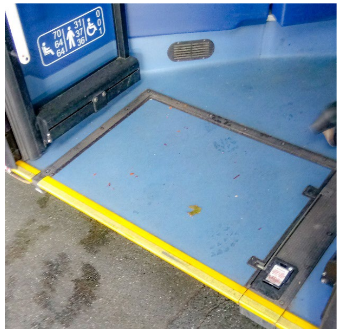
Figure 72. View of disabled ramp undeployed of a 2017 Routmaster bus, Brighton and Hove Bus depot. Personal photograph by Author.01 Nov.2019
