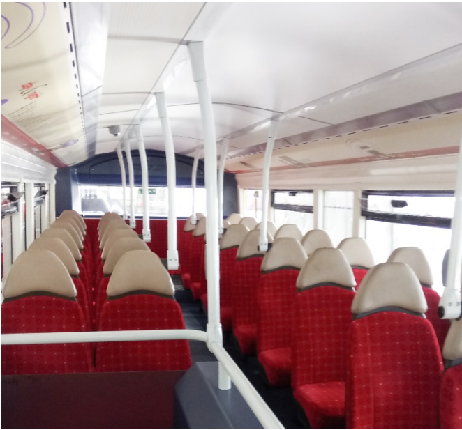
Figure 79. view of upper deck area on a 2017 Routmaster bus showing white grab rails and higher ceilings, Brighton and Hove Bus depot. Personal photograph by Author.01 Nov.2019
