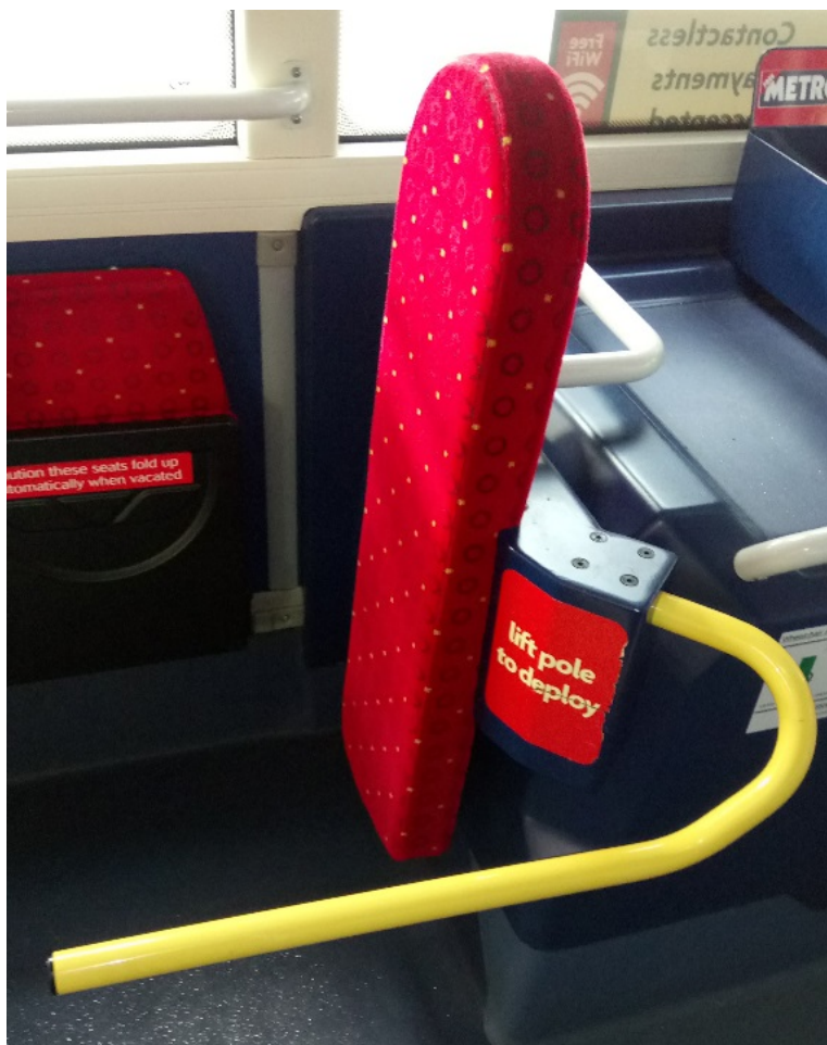
Figure 78. view of wheelchair protective hand rail on a 2017 Routmaster bus, Brighton and Hove Bus depot. Personal photograph by Author.01 Nov.2019
