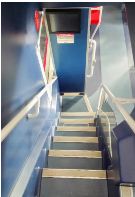
Figure 82 view of stairs to upper deck on a 2017 Routmaster bus, Brighton and Hove Bus depot. Personal photograph by Author.01 Nov.2019
