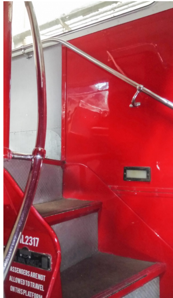
Figure 69. View of narrow, slippery grab handles of a 1965 Routmaster bus, Brighton and Hove Bus depot. Personal photograph by Author.01 Nov.2019
