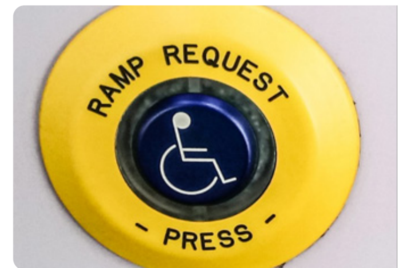
Fig 20: Disabled ramp request button- Brighton and hove Bus Company, 2019- Photo by author.
