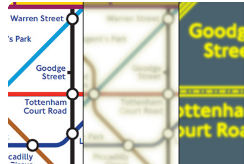
Fig 19: Ian Hamilton : redesign of the London Underground maps for people with visual impairment : How the blue/yellow high contrast version helps those with cataracts. www.brilliantmaps.com/colour-blind-tube-map/
